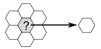
Performing this operation on all the pixels simultaneously results in "noise canceling," which removes isolated black pixels.
