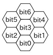
and the binary representation i is defined as  $i = \sum_{j=0}^{6} bit_j \times 2^j$ , where  $bit_j$  is 0 or 1 if the corresponding pixel is in black or white, respectively. Note that the filter is applied on the center pixel, denoted as bit 3.
