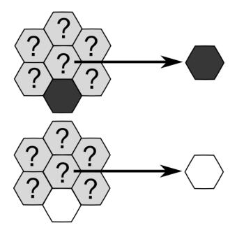
Performing this operation on all the pixels simultaneously results in "shifting up" the whole image by one pixel.
